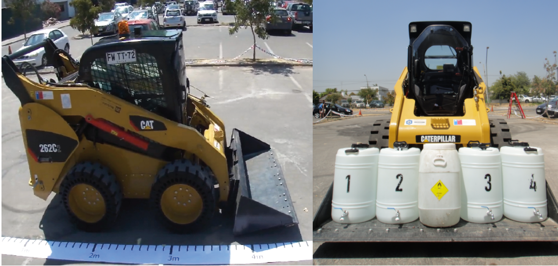
Figure 1: Compact skid-steer loader at the experiment site with unloaded bucket (left) and loaded bucket (right).
